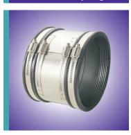
These couplings comply with the requirements of WIS 4-41-01 and are specifically designed for jointing pipes in sewerage, drainage and similar non-pressure applications where resistance to shear loads is required.
