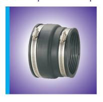
Provide an inexpensive method of directly jointing pipes of differing outside diameters, without the need to use bushes. The most common application is for connecting PVC-u pipes to a variety of other pipe materials including vitrified clay. These couplings are also suitable for connecting other types of pipes including cast iron and metal pipes (up to a maximum outside diameter of 420mm).
